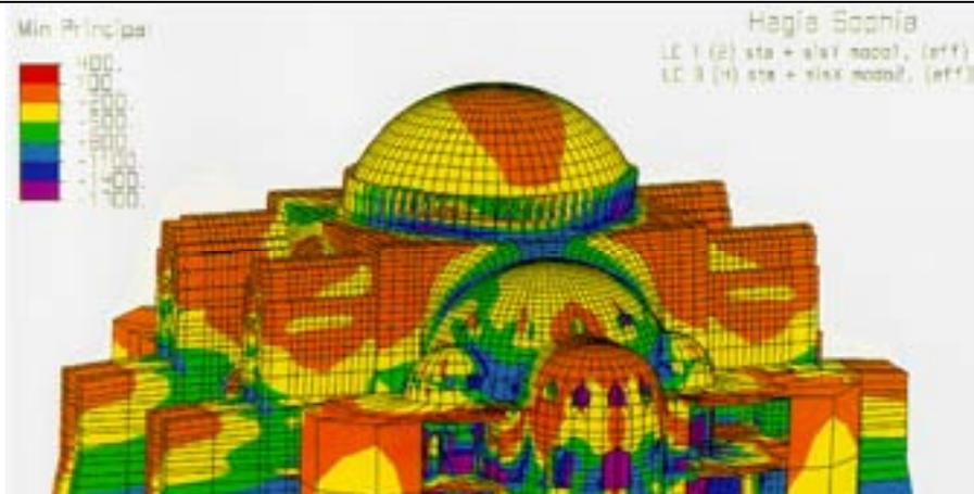
Fig. 21 – Compression stresses produced by an earthquake on the “hemidomes” directions
